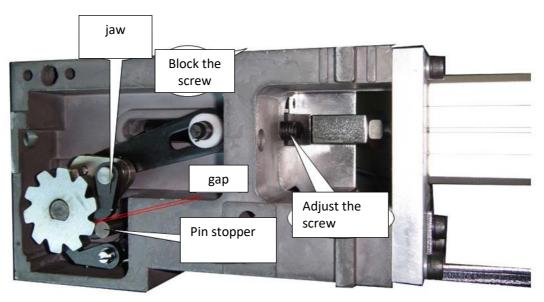
(2). Use a one-word screwdriver to adjust the 0.05-0.1mm gap between the eccentric claw and the ratchet, and lock the plane meter.
