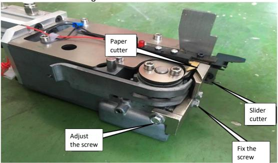
(4). Release the two fixing screws on the retaining main wheel to align the corresponding material foot with the station fork push plate and lock the fixing screw (if 5.0mm, subject to 5.0 on the left).
