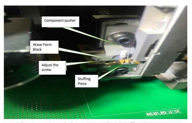
5. Adjust the pusher cylinder to return to the origin. The distance between the pusher fork slope and the chain clamp slope is 1.5 mm.
