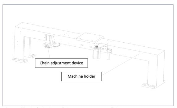
Frame Exploded view of the components of the
