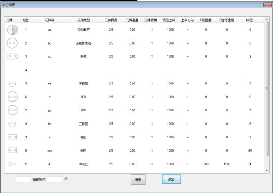
, you can select the component type according to the pin name on the PCB board that is set when the program is made, and set the corresponding component name, and determine the feeding direction. When the component type and loading direction are determined, the 0 degree component schematic image of the Auto Insertion will be displayed in the first column of the list. Please check the schematic image of the changed component on the PCB to ensure that the loading is correct.
