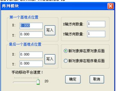
match a certain position in the first module and the same position in the last module, and then enter the number of modules in the X direction and the modules in the Y direction Count, you can generate Auto Insertion data that combines several modules.
