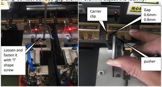
(6). Adjust the cylinder stroke, loosen the cylinder nut, drive the solenoid valve manual switch, so that the material just sent to the chain clip while the element can manually move up and down with a little resistance and no element foot change
