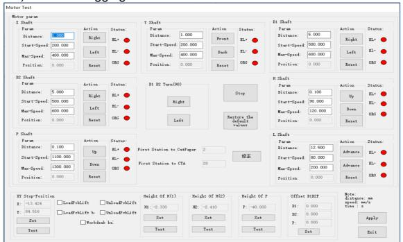
set the movement amount and speed of each axis, and then move each axis according to the direction of the arrow on the button, and test whether the time movement direction of each axis is the same The directions indicated on the arrows are the same; test whether the positive and negative limits are valid and reversed.
