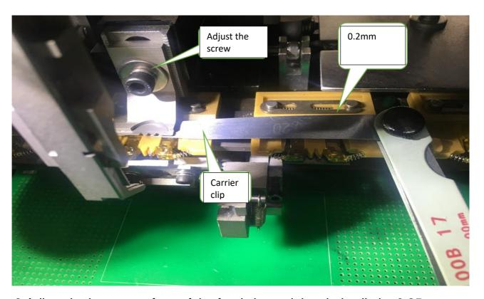
3. Adjust the bottom surface of the feed slot and the chain clip by 0.25 mm, and at the same time make the clip and the feed slot have the same height.
